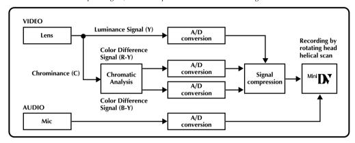
This camcorder separates the data into blocks, writing one block of each data type on each track of the tape.
